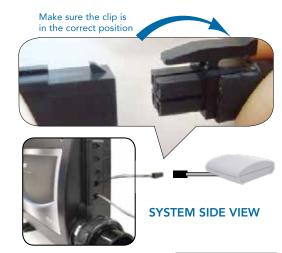
After the Gateway Ultra Spa module is inserted, gently pull on the wire to make sure the clip is securely in place and will not come lose.
